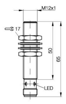
**Inductive Sensors** BES M12MI-NSC20B-S04G M12x1 x 65 normally-open Sn=2mm shielded
